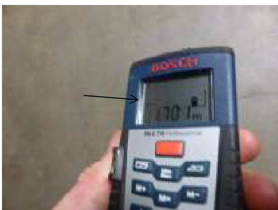
Photograph 15. Bosch electronic distance measure used to record the moisture damage and determine the source of the leak via the design plans.
