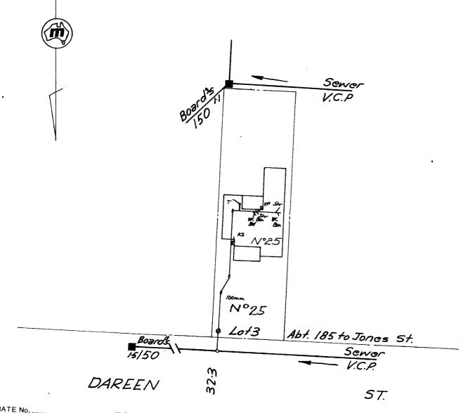
Scale 1 : 500 For House Services Engineer DRAINAGE BRANCH OFFICE .....W.C. Supervised by PLUMBING Date .....Bth. Supervised by Date .....Shr. .....Bsn, Inspector Outfall **N.S.** HL Examined by .....K.s. Inspector .....T. 1407 090 .....Plg. Chief Inspector Plumber..... ੇge, Int. ા. Ext. Tracing Checked..... Boundary Trap
