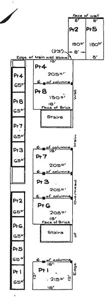
It is intended to limit the height of part lot 2 and part Lot 5 to 8 feet above the concrete floor
