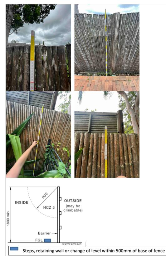
Above is a diagram showing the NCZ5 requirements for an 1800mm boundary fence.
