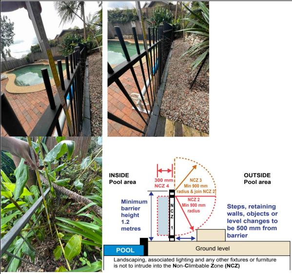
Above is a diagram showing the NCZ requirements for an internal barrier less than 1800mm high.
