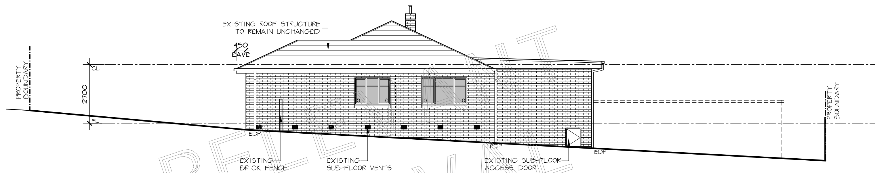
10 EXISTING WEST ELEVATION SCALE 1:100
