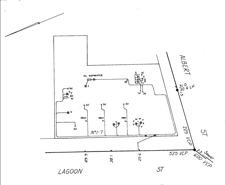
pipe diametres in millimetres Distances/depths in metres Scale: Approx. 1:500
